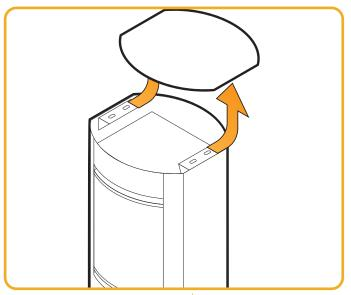
Figure 8.1 | Removing the top cover
