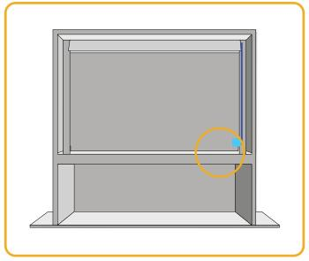
Figure.5.2 | Position of the On/Off switch
