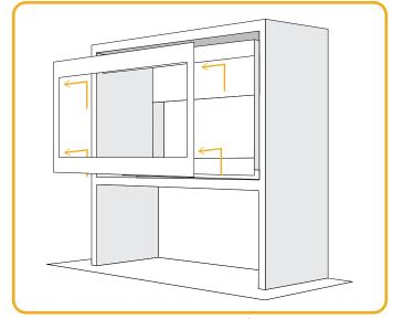
Figure.8.3 | Removing the glass
