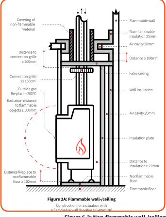
Figure 6-3: Non-flammable wall-/ceiling
