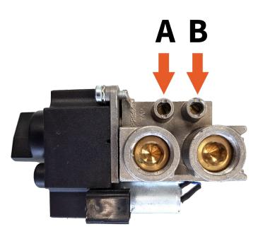
Figure 8-1: measure points on the gas block
