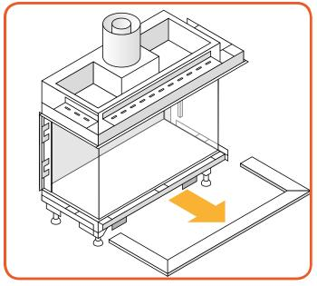
Figure 10-3: Removing the lower trim
