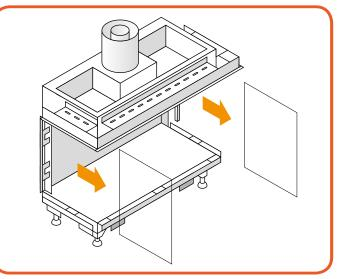
Figure 10-7: Remove side glass (When necessary)
