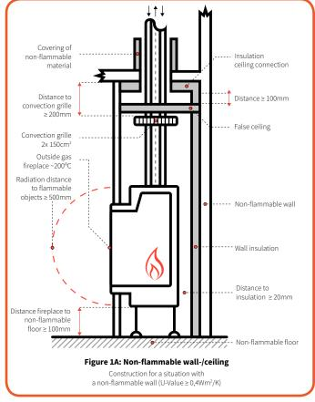
Figure 6-1: Non-flammable wall-/ceiling
