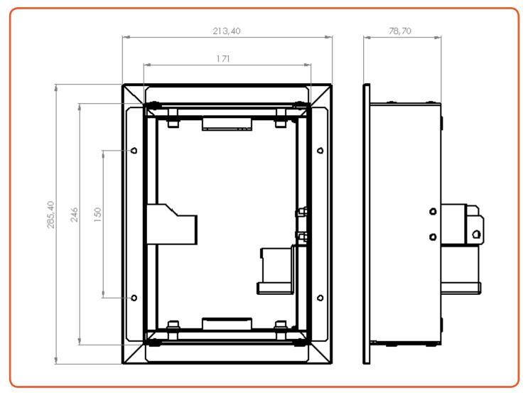
Figure I-1: Service hatch, BDLE4
