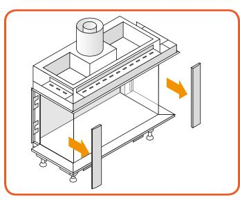
Figure 10-2: Removing side trims
