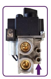
Figure A-4: Testpoint A
