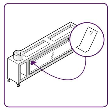
Figure E.1 - Position of the restrictor
