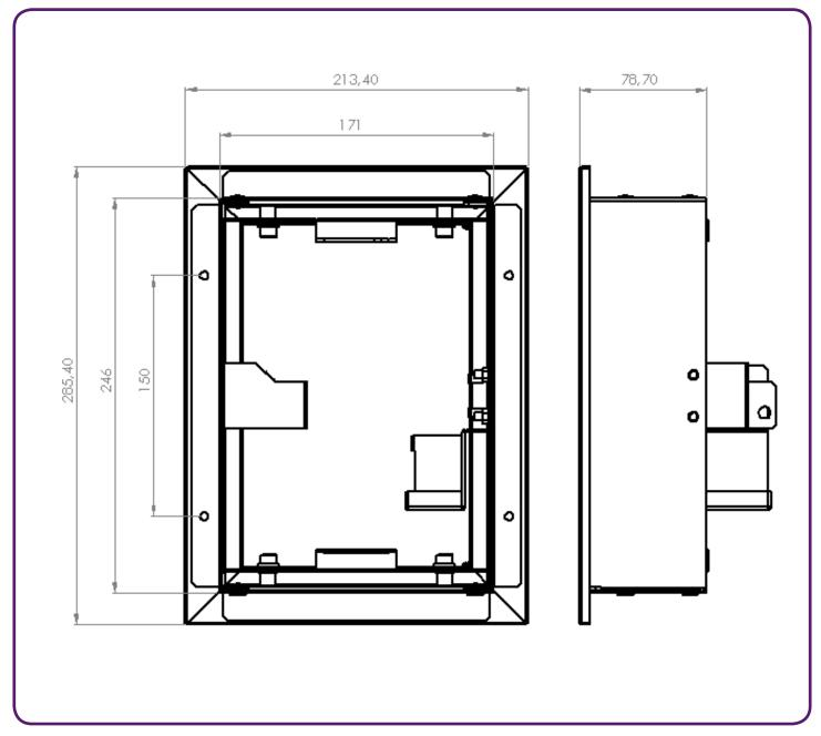
Figure I.1 - Technical drawing of service hatch (BDLE4)
