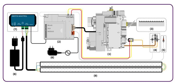
Figure 9.1 - Schematic Electronic Circuit
