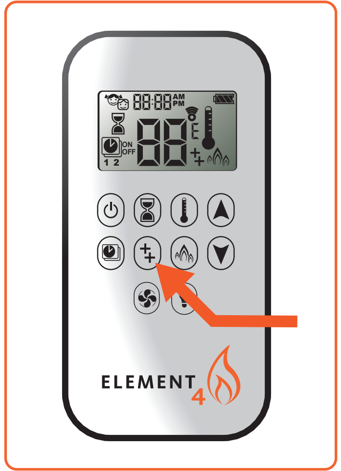
Figure A.L | "Double plus"-button on the remote
