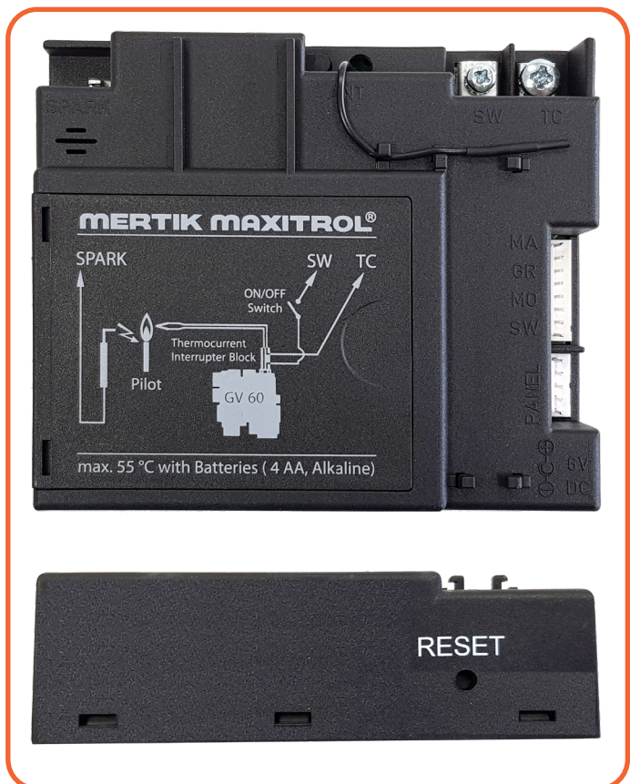
Figure 4.2 | Top and side view of the Receiver
