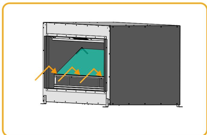
Figure 8.3 | Put the underside of the effect glass in the glass frame
