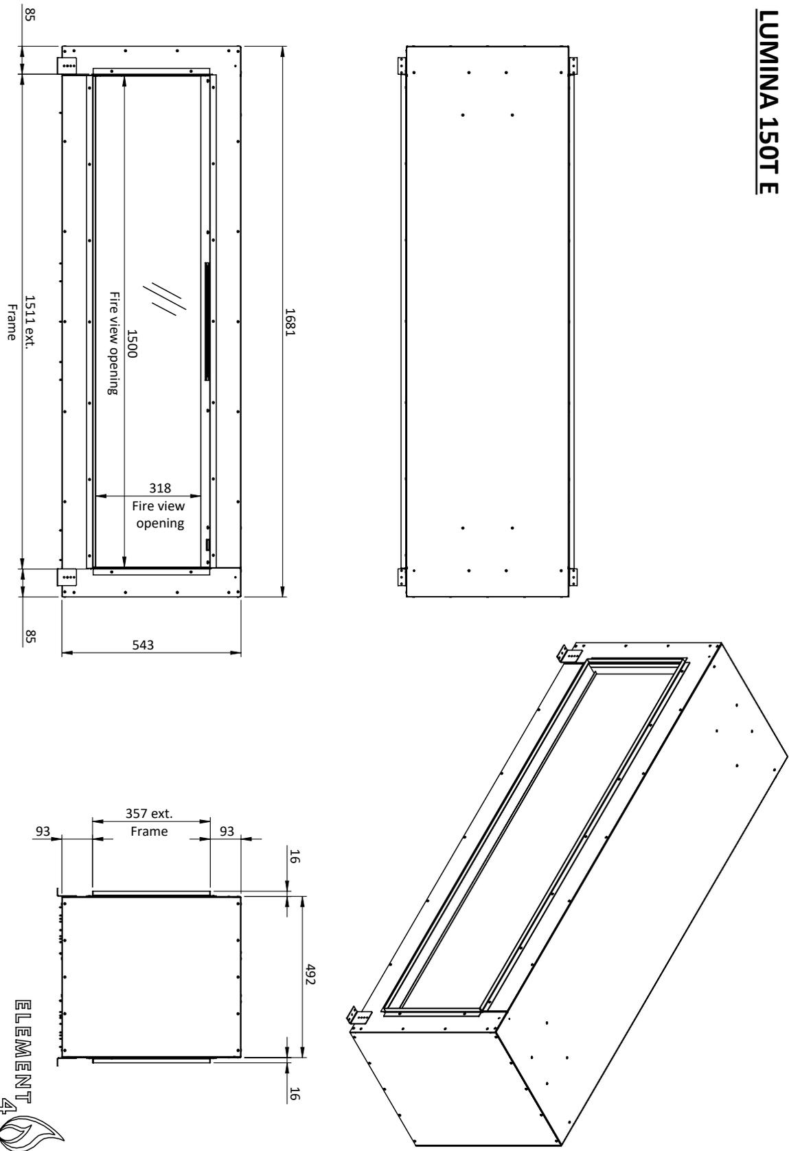
Figure.B.A | Lumina 150T E dimensions
