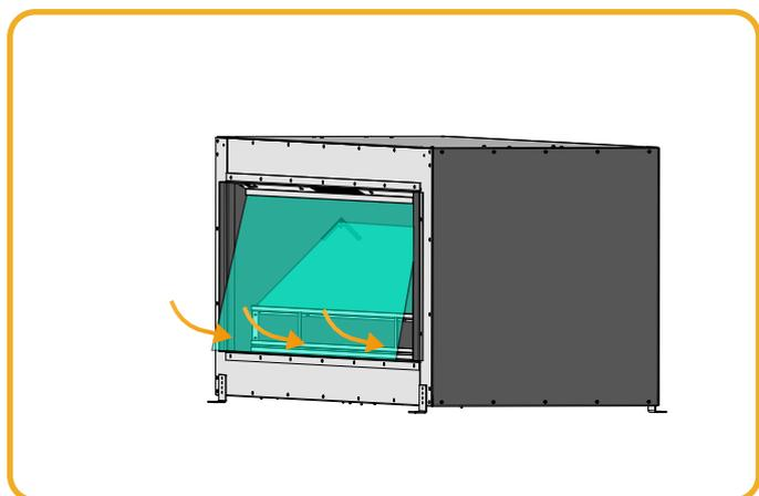
Figure 8.5 | Put the glass in vertical position
