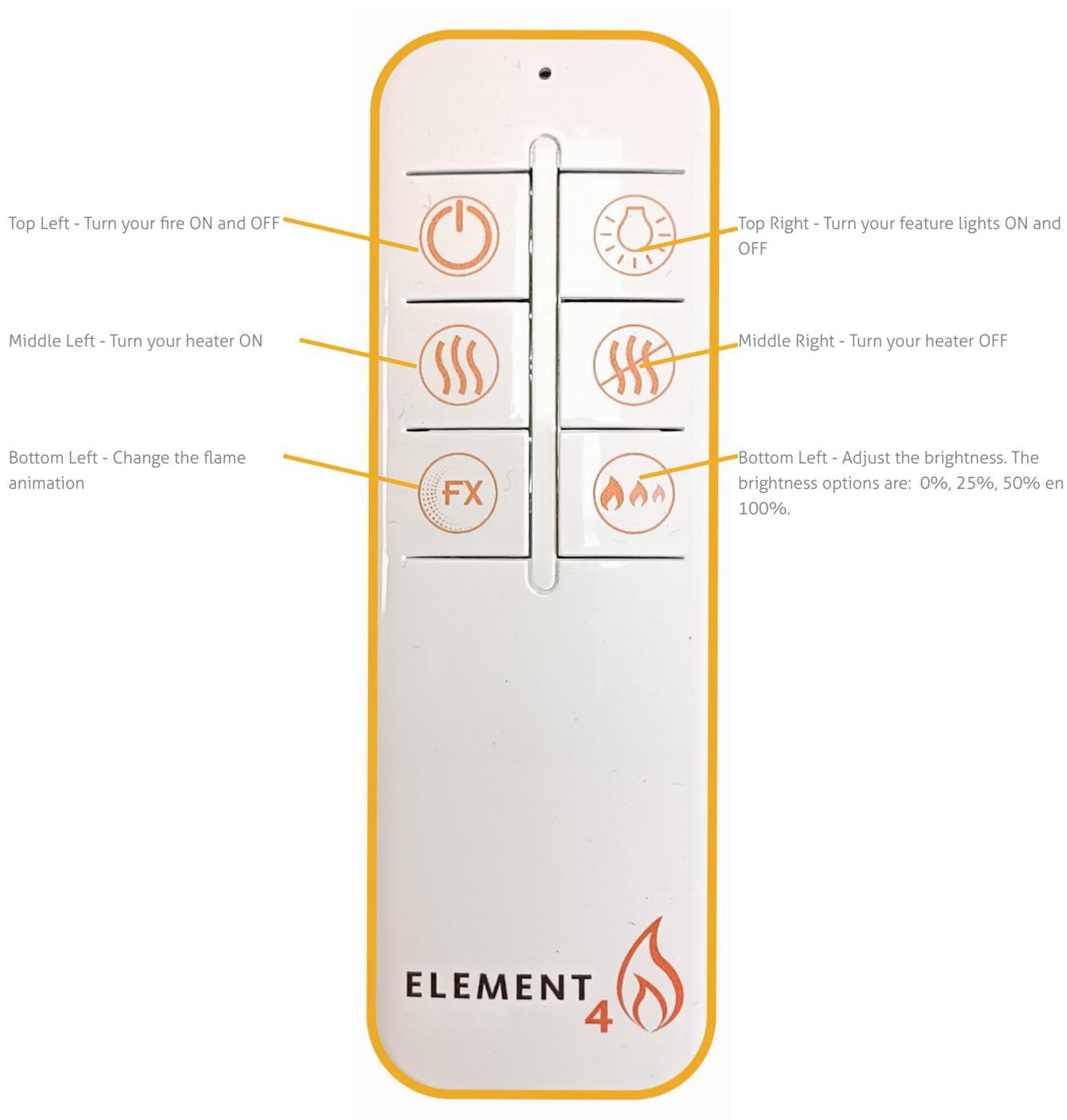
**Attention:** With the remote control the heater is pre-set to 28°. When the temperature inside the fireplace surpasses this the heater will not turn on. If you would like to adjust the temperature, the app should be used.
