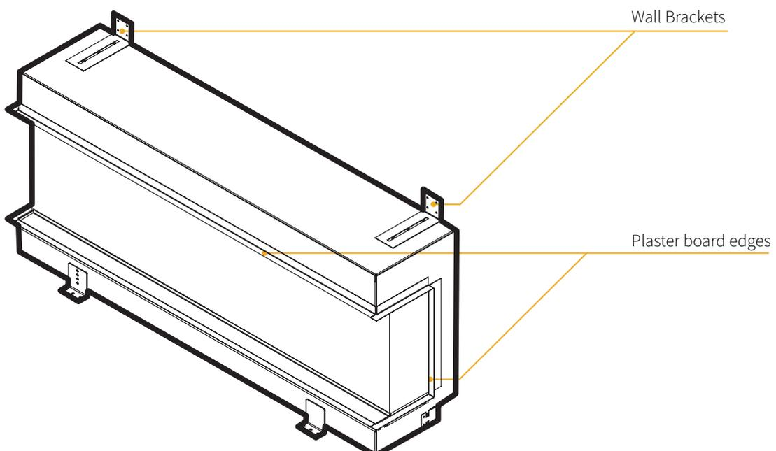
Figure.8.1 | Wall brackets & plaster board locations
