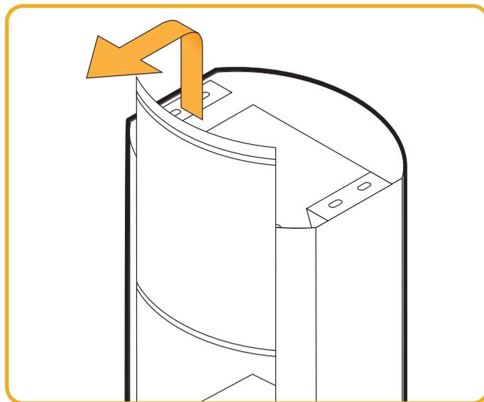
Figure 8.3 | Remove the glass vertically
