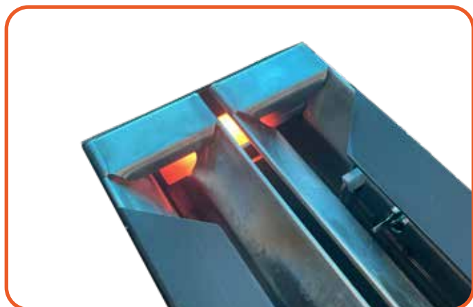
Figure. 4.5 PRIMING: Fuel is going to be ignited
