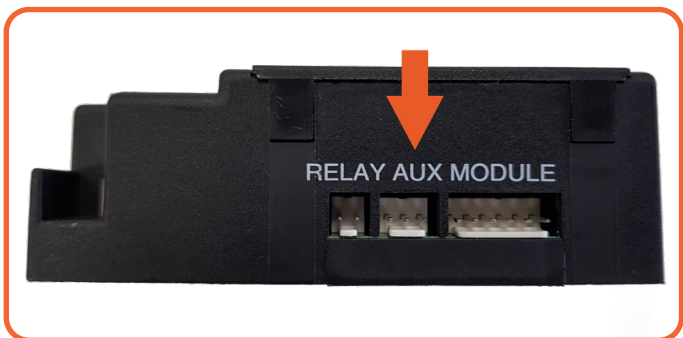
Figure A.K | Aux-position receiver
