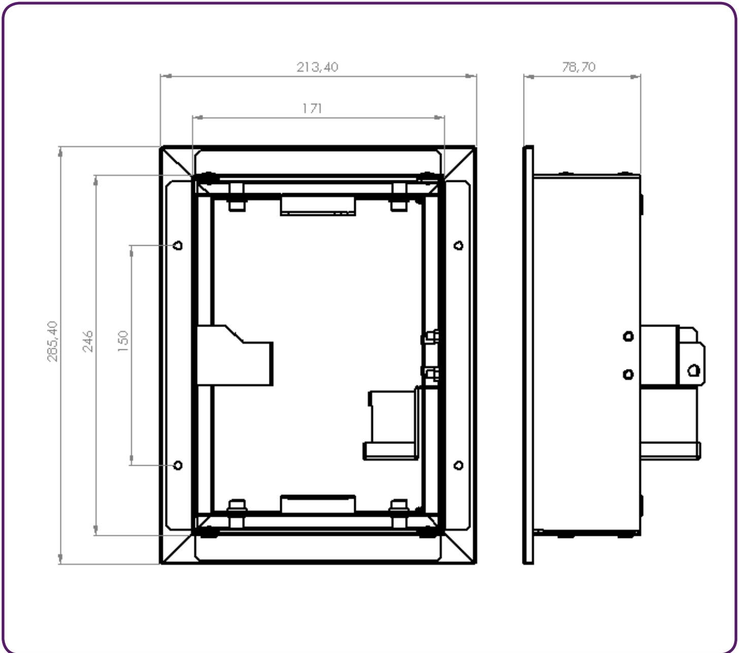
Figure I.1 - Technical drawing of service hatch (BDLE4)
