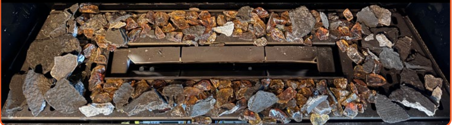
Fill the remaining open areas with black chips. Use smaller chips to put on top of the amber glass. Ensure that no chips fall into the burner.
