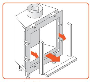
Figure 9.4  $\mid$  Remove side and bottom trims
