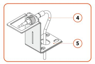
Figure 9.11 | Isometric drawing of second thermocouple
