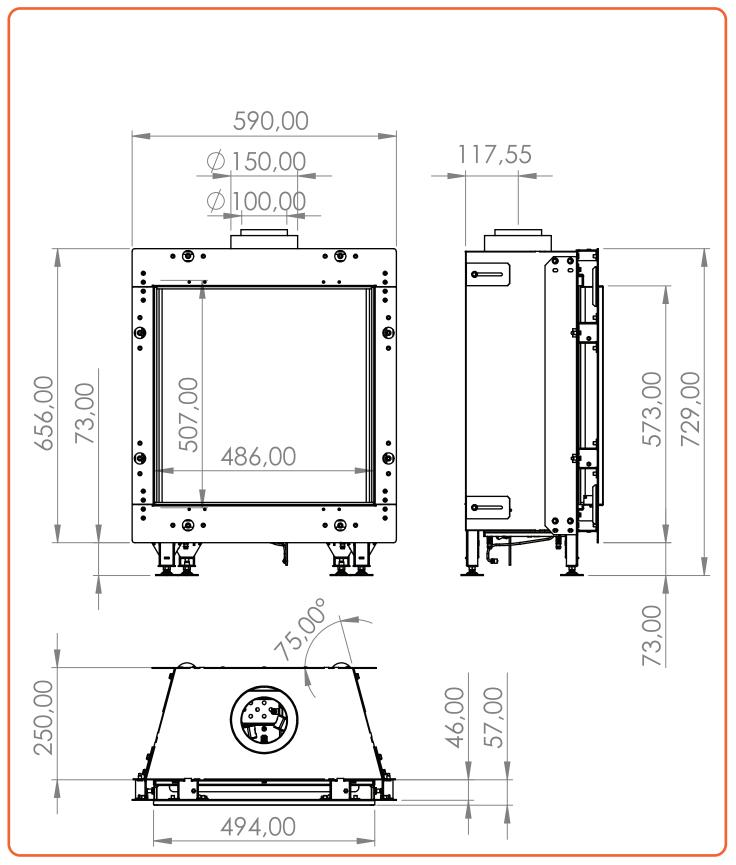
Figure H.B | Technical drawing of Cupido 50
