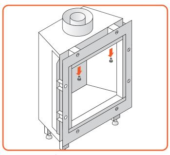
Figure 9.2  $\mid$  Remove screws from the upper trims
