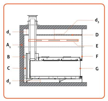
Figure 6.1 | C11: Flue situation Non-Flammable materials
