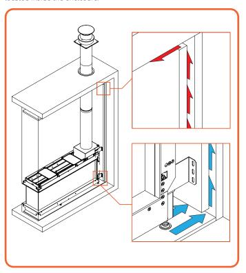
Figure 6.5 | Air flow between wall covers
