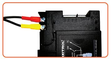
Figure A.F | Wiring receiver
