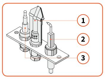
Figure 9.10 | Isometric drawing of the pilot set
