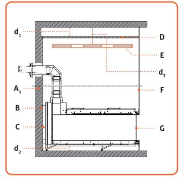
Figure 6.2 | C31: Flue situation Non-Flammable materials
