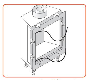
Figure 9.5 | Remove glas rope
