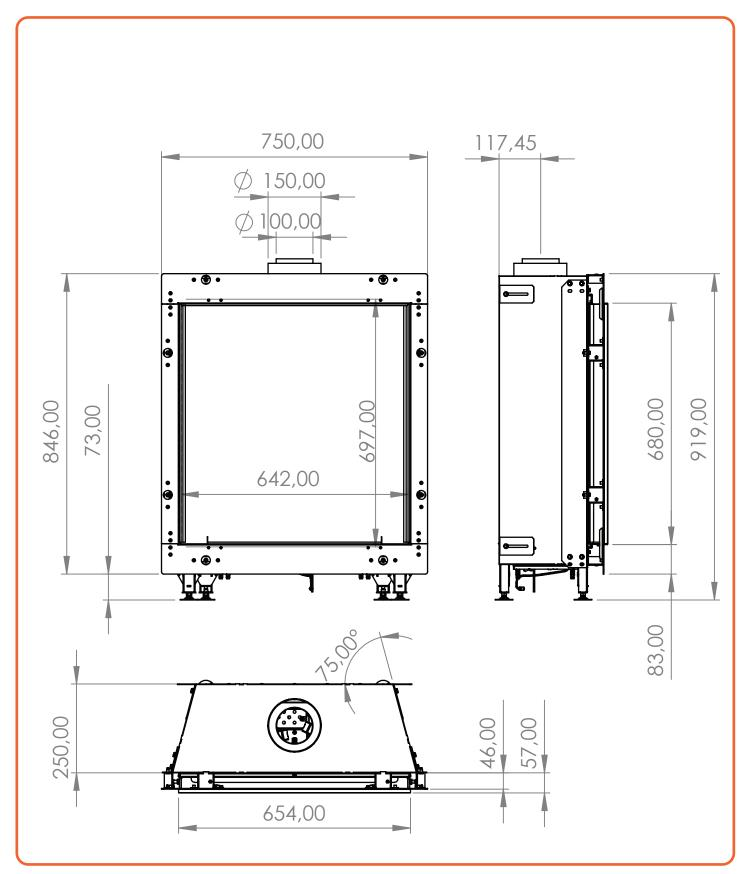
Figure H.A | Technical drawing of the Cupido 70
