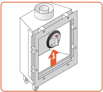
Figure 9.6 | Put on suction cup and lift a bit
