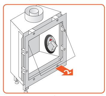
Figure 9.7 | Carefully tilt out the glass
