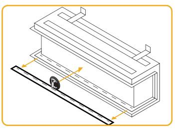
Figure.9.3 | Remove second glass retainer strip
