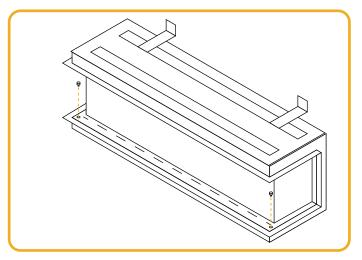
Figure.9.1 | When present: remove bottom screws
