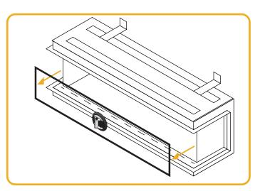
Figure.9.4 | Carefully remove the glass
