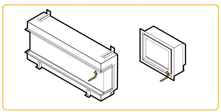
Figure.5.1 Positions of the On/Off switches
