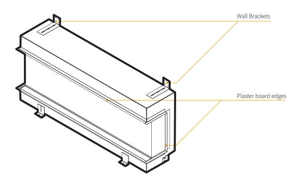
Figure.8.1 | Wall brackets & plaster board locations
