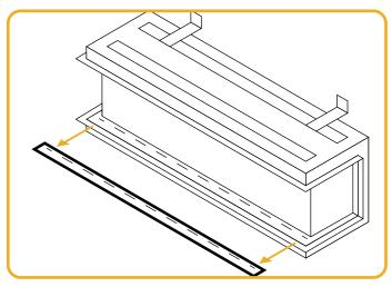
Figure.9.2 | Remove glass retainer strip
